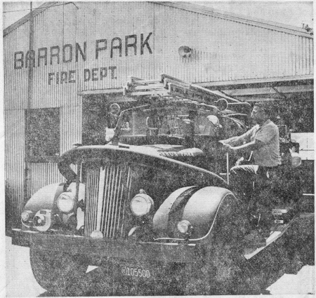
OLD-TIMERS—Anthony Musachia, Barron Park's first and only volunteer fire chief, warms up his department's 1949 Van Pelt pumper in front of aluminum-walled fire station tucked behind a flower stand on El Camino Real. —Staff Photos
